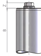
BC: flat top with vent plug G
