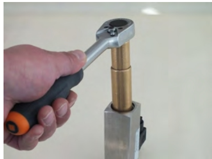
Fig. 51: Loosen threaded ring (inlet)
