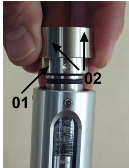
Fig. 49: Position process connection (outlet) in device housing
