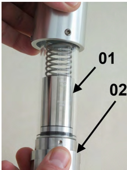
Fig. 37: Remove inner section
