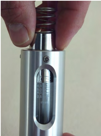
Fig. 48: Insert float and inner parts
