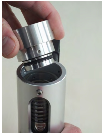
Fig. 35: Remove the process connection (outlet)
