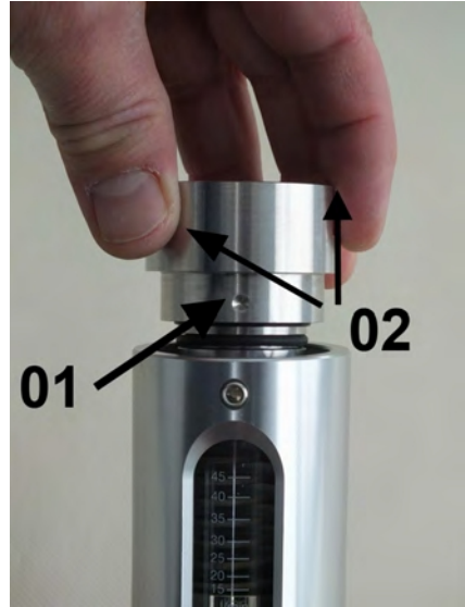
Fig. 49: Position process connection (outlet) in device housing
