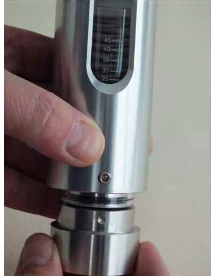
Fig. 45: Insert the process connection into the device housing
