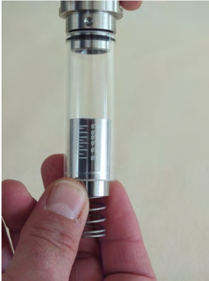
Fig. 38: Remove float, magnets and spring
