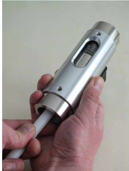
Fig. 51: Check for free movement
