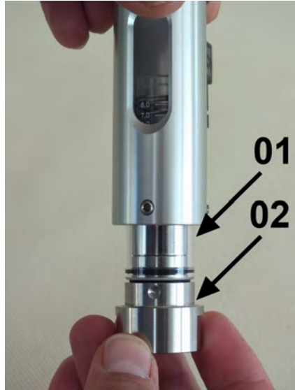
Fig. 37: Remove the inner section
