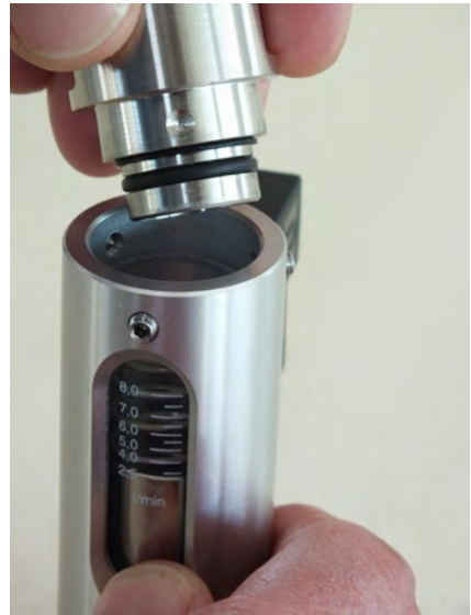
Fig. 35: Remove the process connection (outlet)
