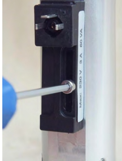
Fig. 32: Loosen fixing screw
