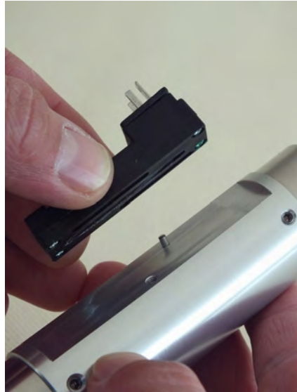
Fig. 55: Remove switch housing
