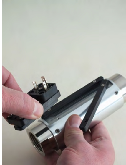
Fig. 57: Remove switch contact
