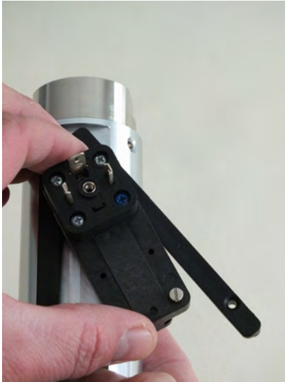
Fig. 56: Rotate guide rail to the side
