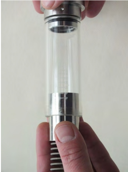
Fig. 38: Remove float, magnets and spring
