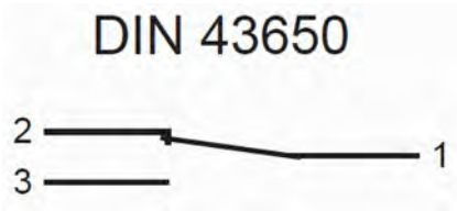
Fig. 15: Switch position under no-flow condition
