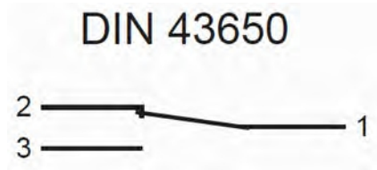
Fig. 16: Switch position under no-flow condition
