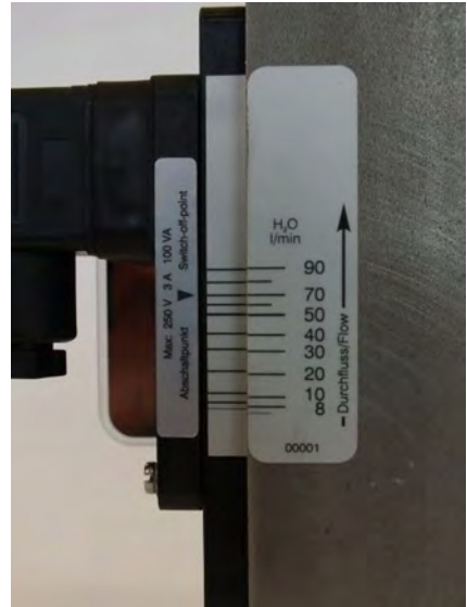
Fig. 4: SW-06 switch point adjustment scale
