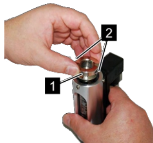
Fig. 54: Position the outlet process connection
