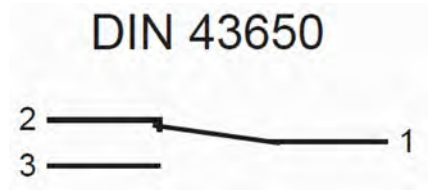
Fig. 15: Switch position under no-flow condition
