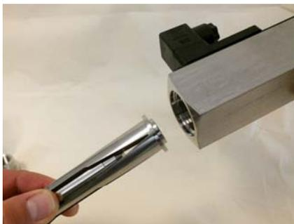
*Fig. 36: Remove inner parts*
