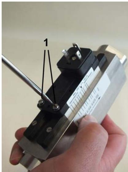
Fig. 52: Loosen set screws
