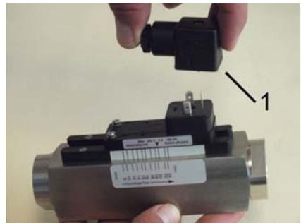
Fig. 20: Remove socket
