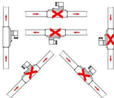
Fig. 5: Installation position/direction of flow
