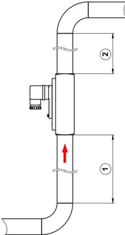
Fig. 6: Unimpeded flow sections
