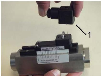
Fig. 51: Remove female socket
