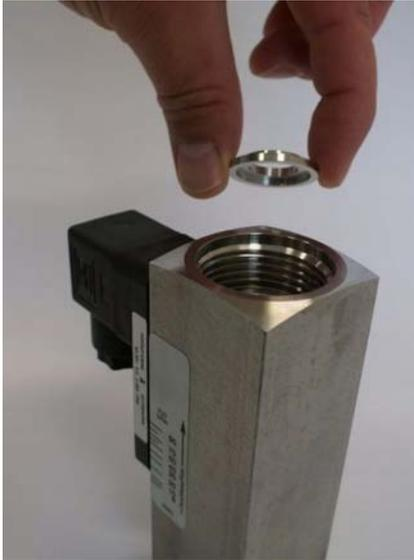
Fig. 36: Remove the centering disc (outlet)
