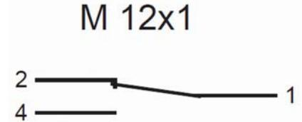
Fig. 19: Switch position under no-flow condition
