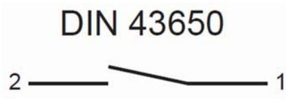
Fig. 13: Switch position under no-flow condition
