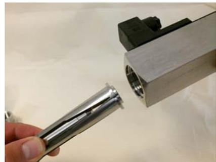
Fig. 45: Insert inner parts
