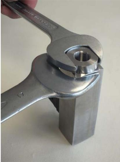
Fig. 43: Tighten process connection (inlet)
