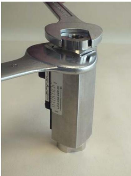
*Fig. 34: Loosen process connection (outlet)*
