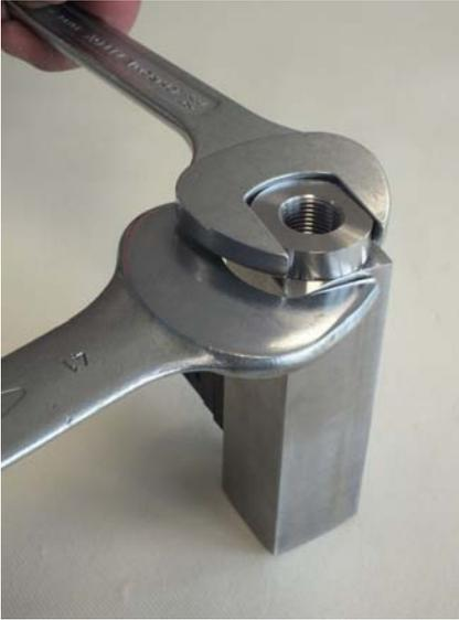
Fig. 44: Tighten process connection (inlet)
