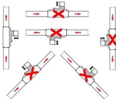
*Fig. 5: Installation position/direction of flow*
