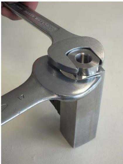
*Fig. 39: Loosen process connection (inlet)*
