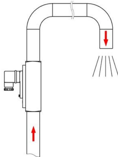
Fig. 7: Unimpeded outlet
