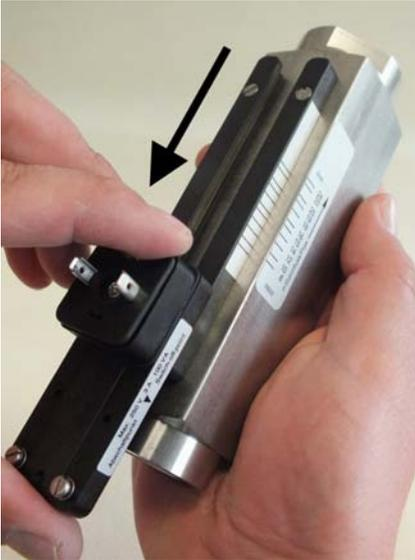
*Fig. 54: Remove the switch contact from guide rails*
