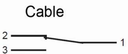
Switch position under no-flow condition
