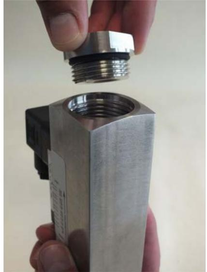
*Fig. 48: Insert process connection (outlet)*
