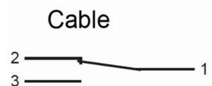
Switch position under no-flow condition
