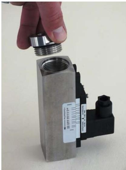
*Fig. 40: Remove the process connection (inlet)*
