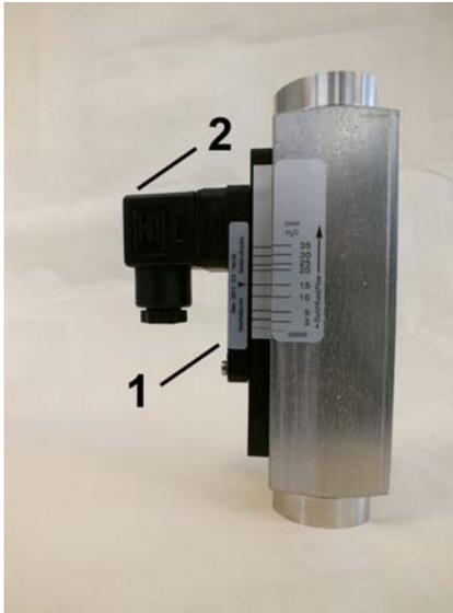
*Fig. 3: Switch contact and female socket*
