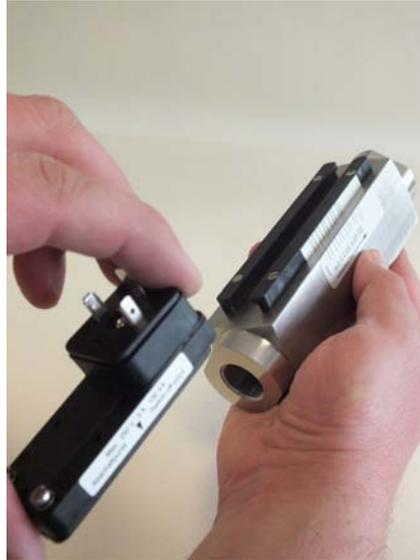
*Fig. 55: Remove switch contact*
