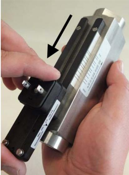
*Fig. 53: Remove the switch contact from guide rails*
