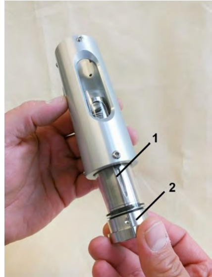
Fig. 38: Remove the inner section
