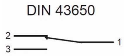
Fig. 14: Switch position under no-flow condition
