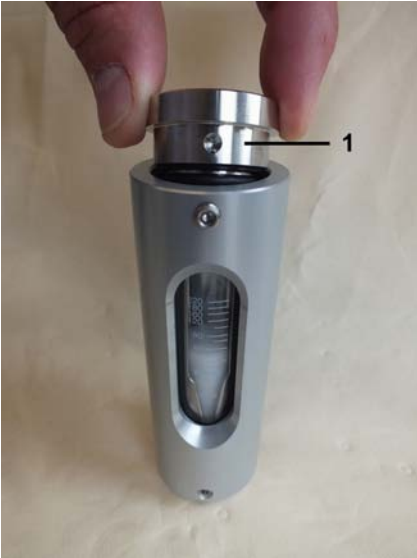
Fig. 52: Position the outlet process connection
