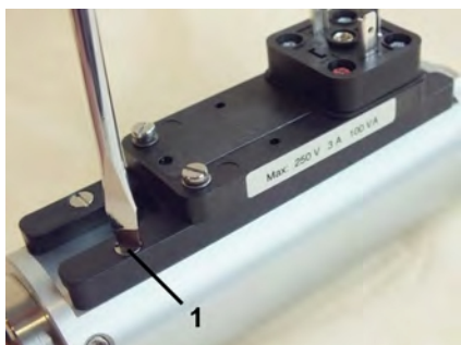
Fig. 59: Release the guide rail
