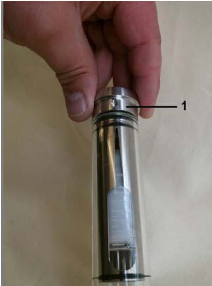
Fig. 46: Process connection (Inlet)
