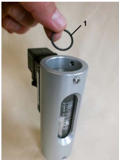
Fig. 35: Slot nozzle buffer O-ring
