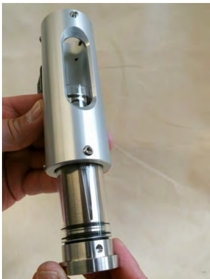
Fig. 49: Insert the process connection into the device housing
