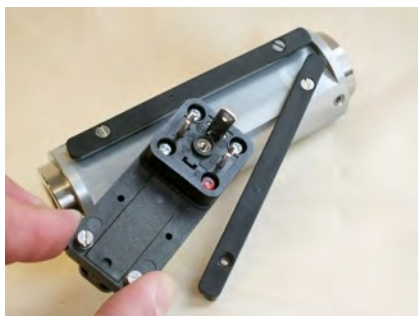
Fig. 61: Remove switch contact
