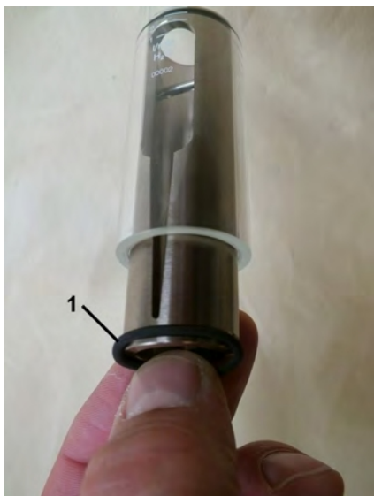
Fig. 45: Centering the slot nozzle
