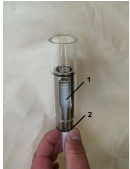
Fig. 44: Insert slot nozzle
