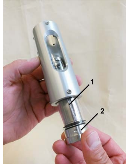
Fig. 37: Remove the inner section
