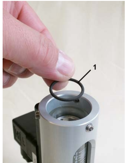
Fig. 51: O-ring, slot nozzle buffer
