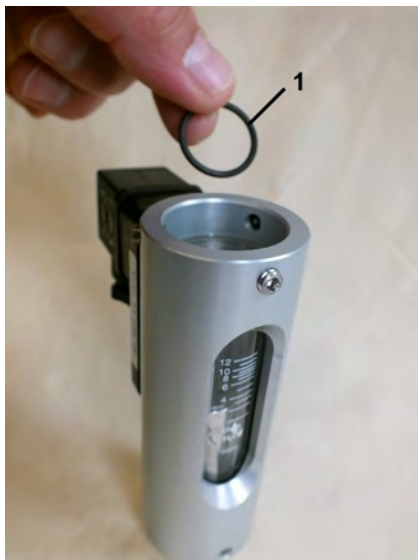
Fig. 36: Slot nozzle buffer O-ring
