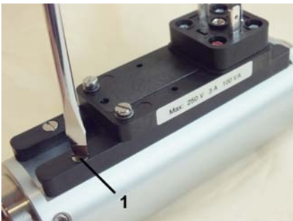
Fig. 58: Release the guide rail
