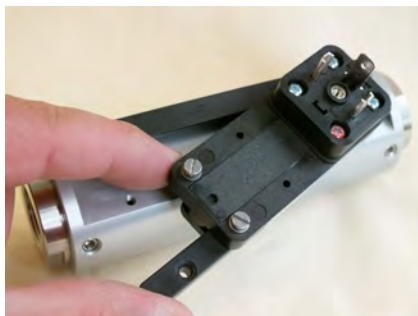
Fig. 60: Rotate guide rail to the side
