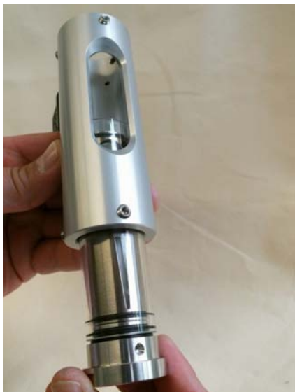
Fig. 48: Insert the process connection into the device housing
