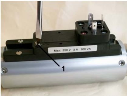
Fig. 57: Loosen set screws
