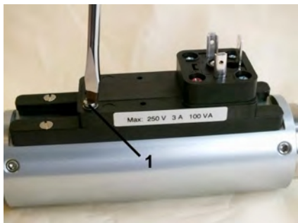
Fig. 58: Loosen set screws
