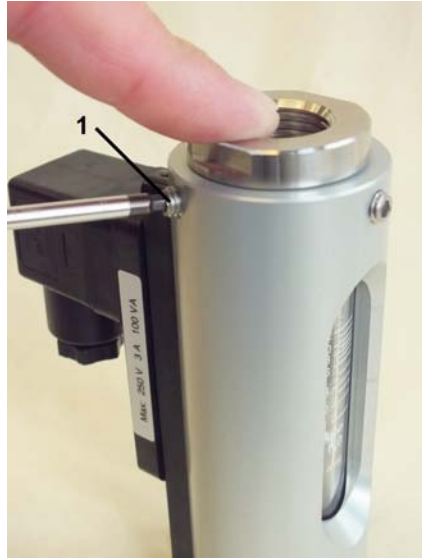
Fig. 53: Tighten hex socket screws
