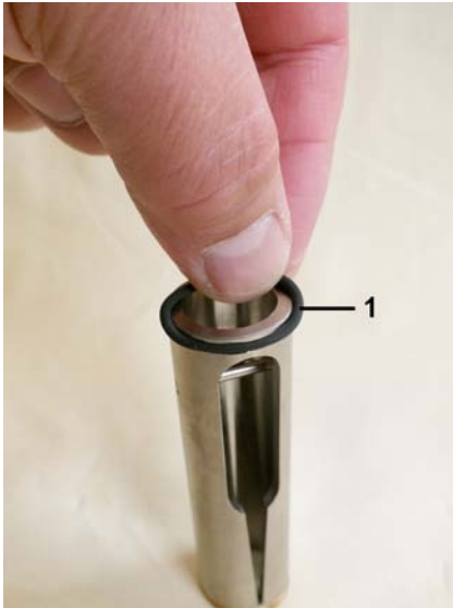
Fig. 42: O-ring (centering the slot nozzle)
