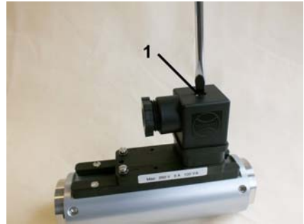
Fig. 55: Loosen female socket
