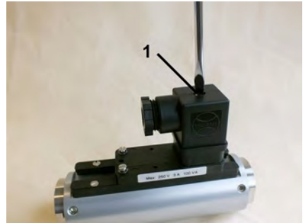
Fig. 56: Loosen female socket
