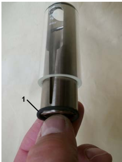
Fig. 44: Centering the slot nozzle
