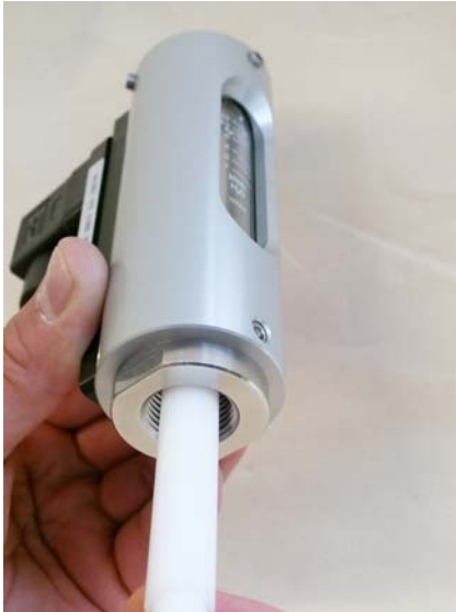
Fig. 54: Check for free movement
