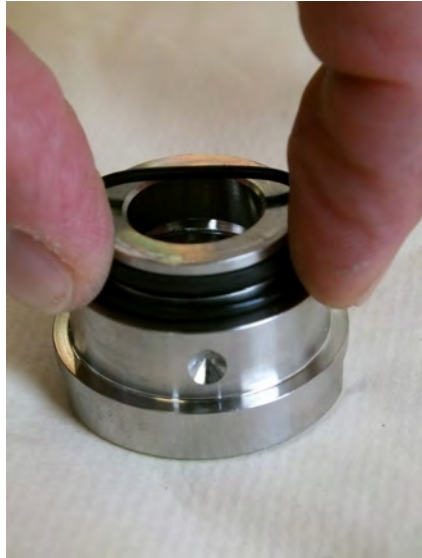
Fig. 41: O-ring (glass buffer)
