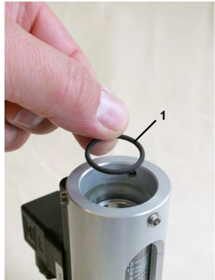
Fig. 52: Slot nozzle buffer
