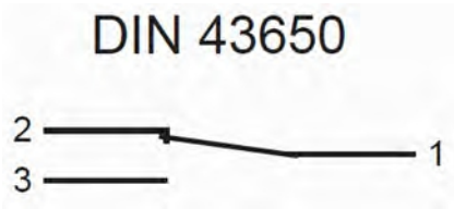
Fig. 15: Switch position under no-flow condition
