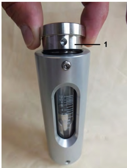
Fig. 53: Position the outlet process connection
