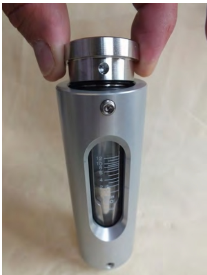
Fig. 35: Remove the process connection (outlet)
