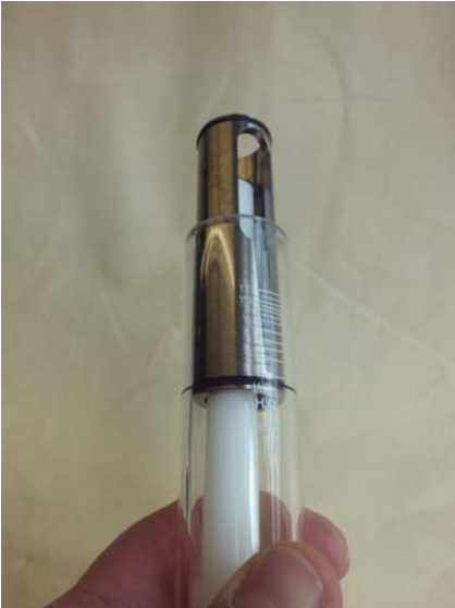
Fig. 38: Remove slot nozzle
