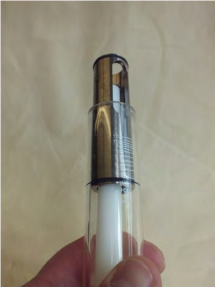
Fig. 39: Remove slot nozzle
