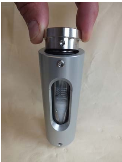
Fig. 34: Remove the process connection (outlet)
