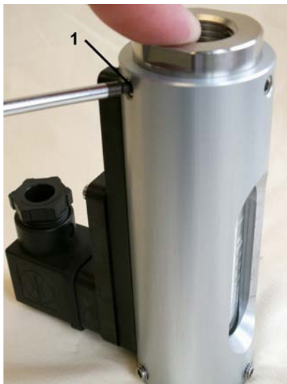
Fig. 49: Secure the process connection (inlet)
