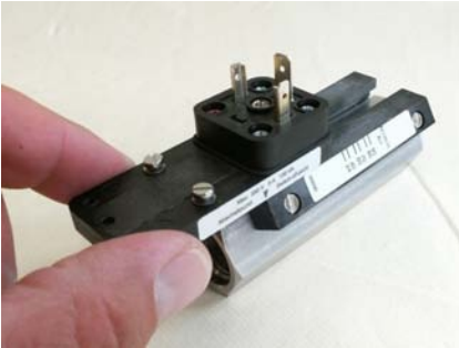
Fig. 46: Remove switch contact from guide rails
