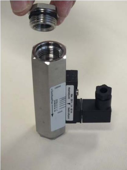
Fig. 42: Remove the process connection (inlet)
