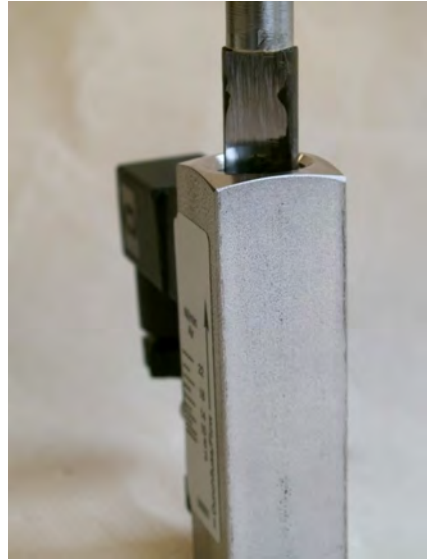
Fig. 35: Loosen threaded ring (outlet)
