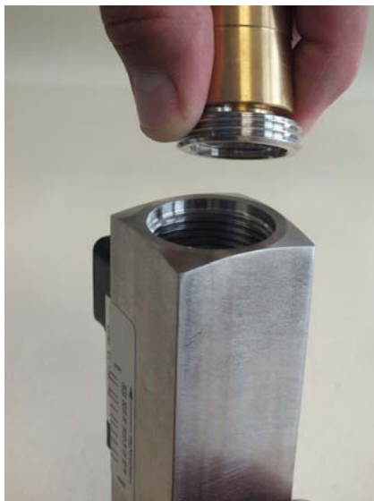
Fig. 37: Remove threaded ring (outlet)
