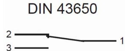
Fig. 15: Switch position under no-flow condition
