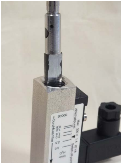
Fig. 43: Seat threaded ring (inlet)
