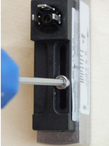
Fig. 32: Loosen the set screw
