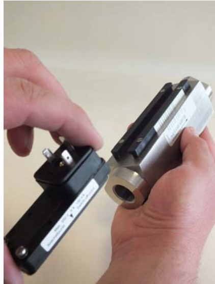
Fig. 62: Remove switch contact
