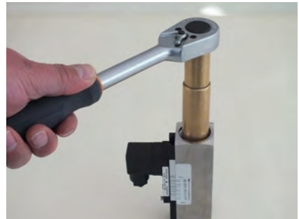
Fig. 55: Seat threaded ring (outlet)
