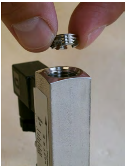
Fig. 46: Insert threaded ring (outlet)
