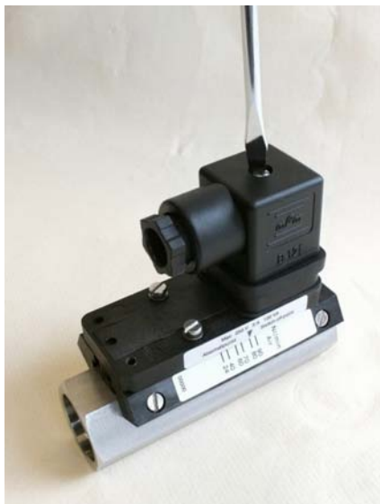
Fig. 43: Loosen female socket
