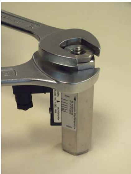
Fig. 52: Tighten process connection (outlet)
