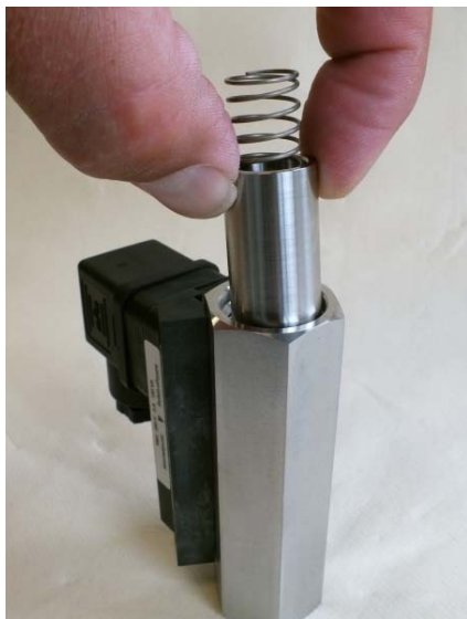
Fig. 39: Insert inner parts
