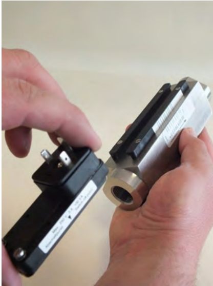
Fig. 63: Remove switch contact
