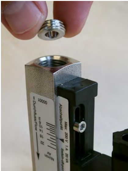
Fig. 41: Remove threaded ring (inlet)
