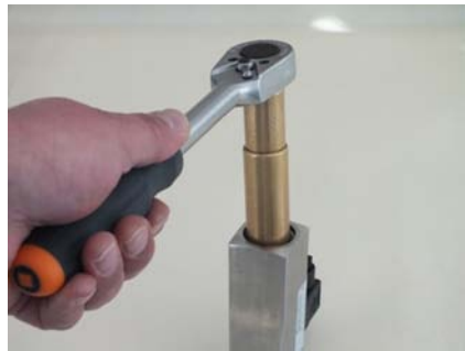
Fig. 48: Seat threaded ring (inlet)
