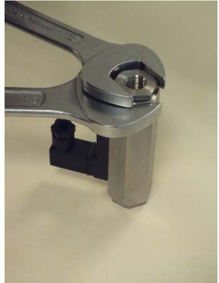
Fig. 46: Tighten process connection (inlet)
