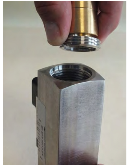
Fig. 38: Remove threaded ring (outlet)
