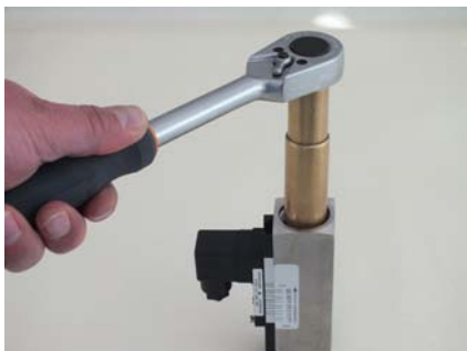
Fig. 36: Loosen threaded ring (outlet)
