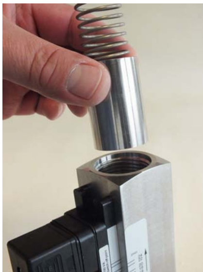
Fig. 52: Insert inner parts
