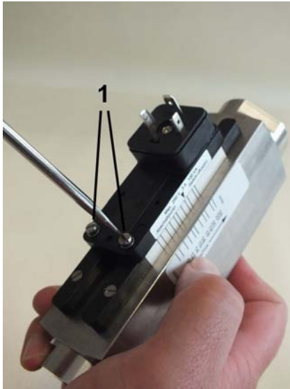
Fig. 31: Loosen the set screws
