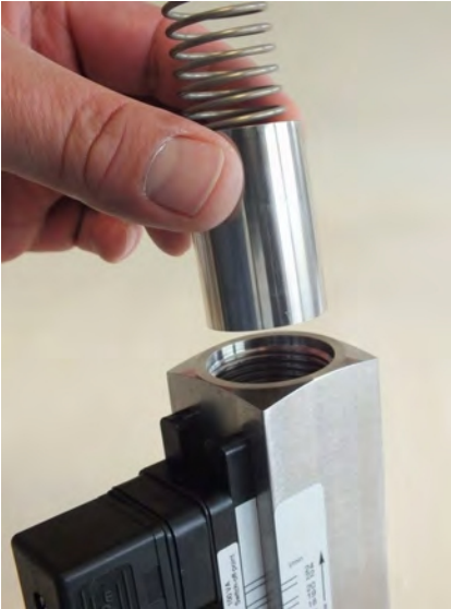
Fig. 53: Insert inner parts
