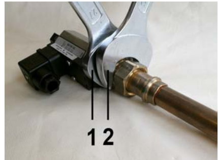
Fig. 11: Screw in the device
