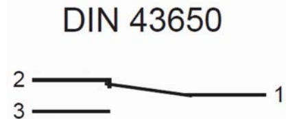
Fig. 15: Switch position under no-flow condition
