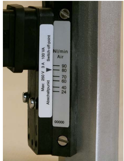
Fig. 4: Switch point adjustment scale SW-02.2
