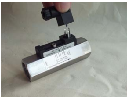
Fig. 55: Remove female socket
