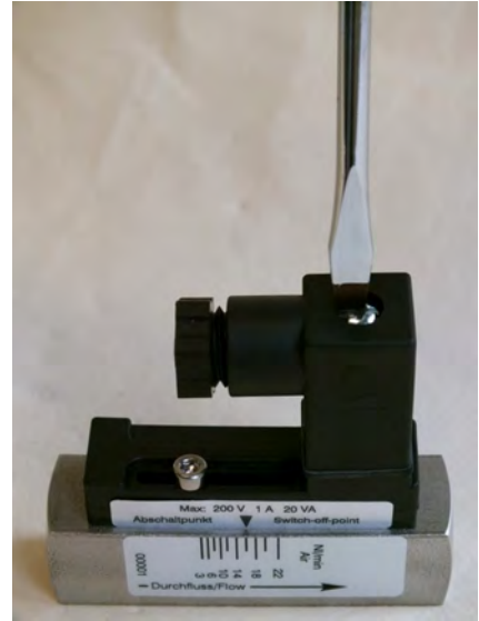
Fig. 49: Loosen female socket
