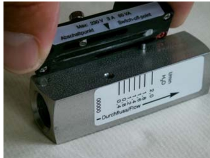
Fig. 52: Remove switch contact
