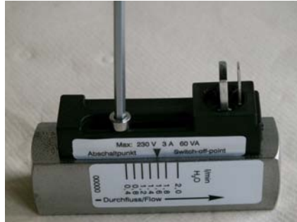
Fig. 51: Loosen set screw
