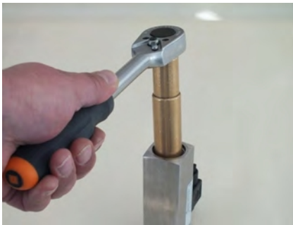
Fig. 49: Seat threaded ring (inlet)
