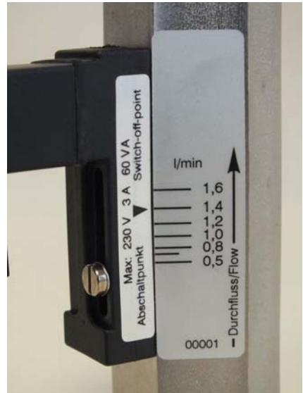
Fig. 4: Switch point adjustment scale
