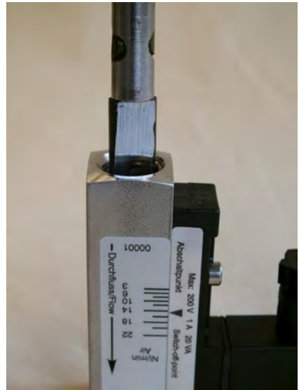
Fig. 40: Loosen threaded ring (inlet)
