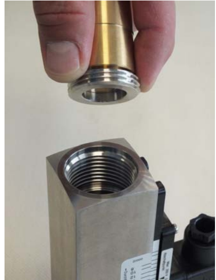
Fig. 44: Remove threaded ring (inlet)
