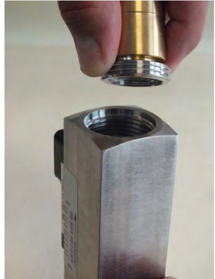
Fig. 54: Insert threaded ring (outlet)
