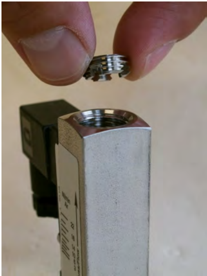
Fig. 36: Remove threaded ring (outlet)
