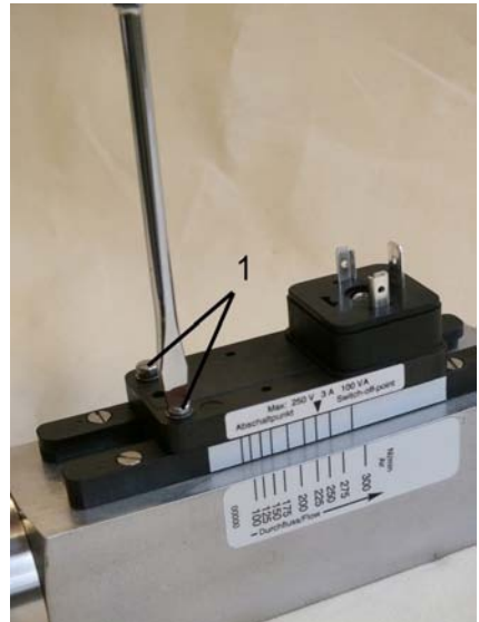
Fig. 60: Loosen set screws
