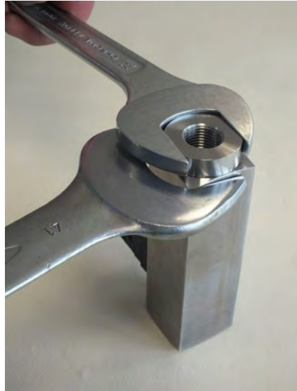
Fig. 41: Loosen process connection (inlet)
