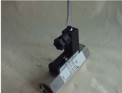
Fig. 54: Loosen female socket
