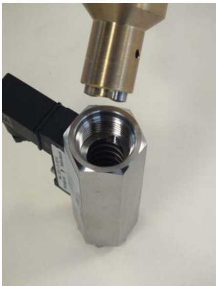
Fig. 36: Insert threaded ring insertion tool (outlet)
