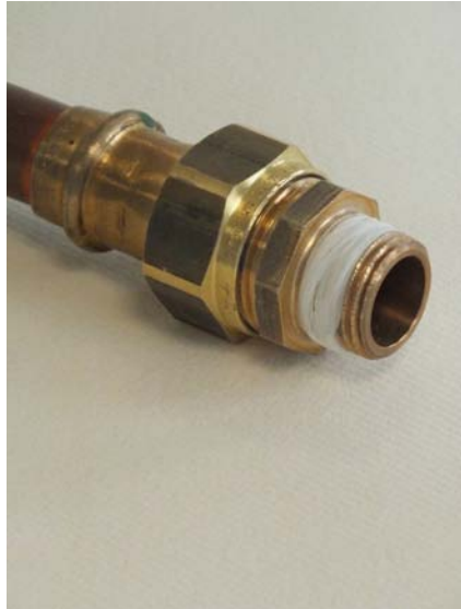
Fig. 9: Pipe connection with sealing thread
