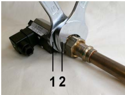
Fig. 10: Screw in the device
