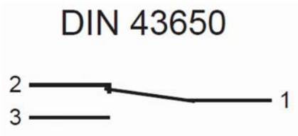
Fig. 14: Switch position under no-flow condition
