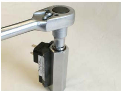
Fig. 34: Loosen threaded ring (outlet)
