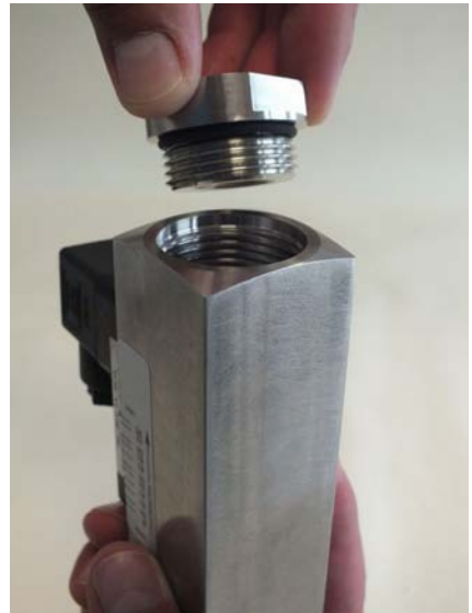
Fig. 55: Insert process connection (outlet)
