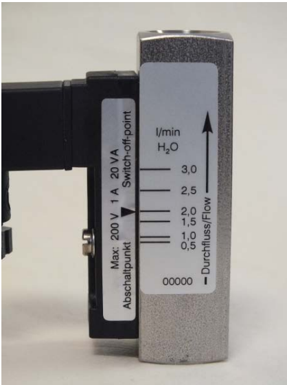
Fig. 33: Reading-off the flow value (sample scale)
