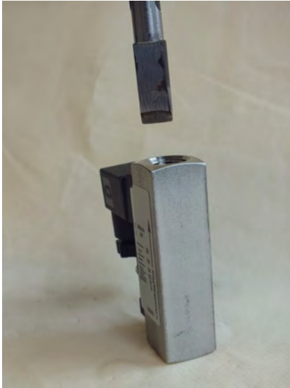
Fig. 34: Insert threaded ring insertion tool (outlet)
