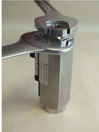
Fig. 57: Tighten process connection (outlet)
