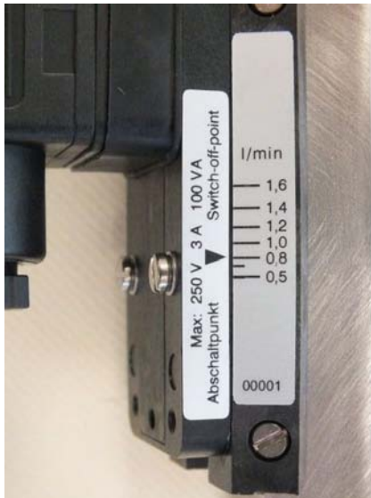
Fig. 32: Reading-off the switch point value
