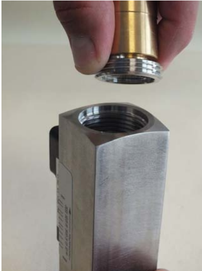
Fig. 53: Insert threaded ring (outlet)
