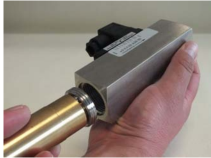
Fig. 47: Insert threaded ring (inlet)
