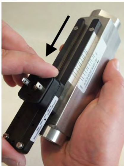
Fig. 62: Remove switch contact from guide rails
