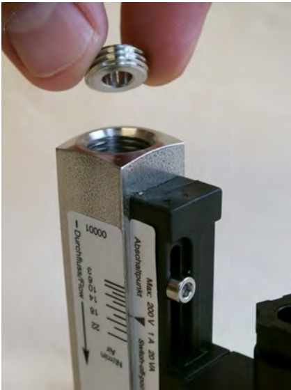
Fig. 42: Insert threaded ring (inlet)
