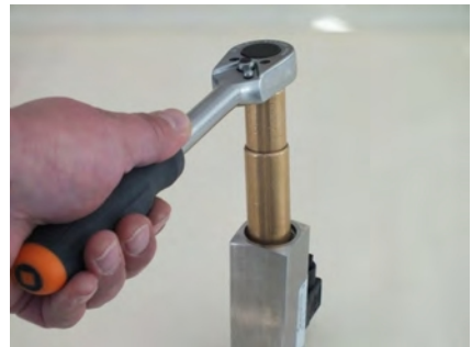
Fig. 44: Loosen threaded ring (inlet)
