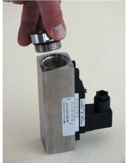
Fig. 50: Insert process connection (inlet)
