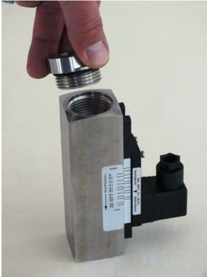
Fig. 42: Remove the process connection (inlet)
