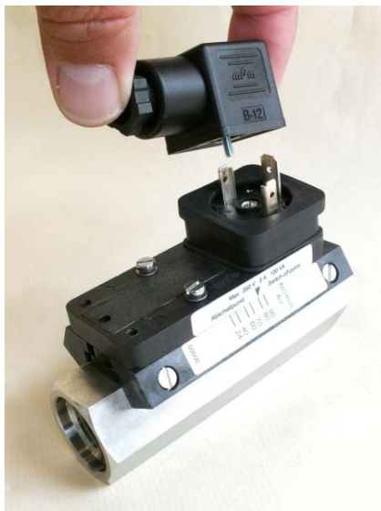
Fig. 44: Remove female socket
