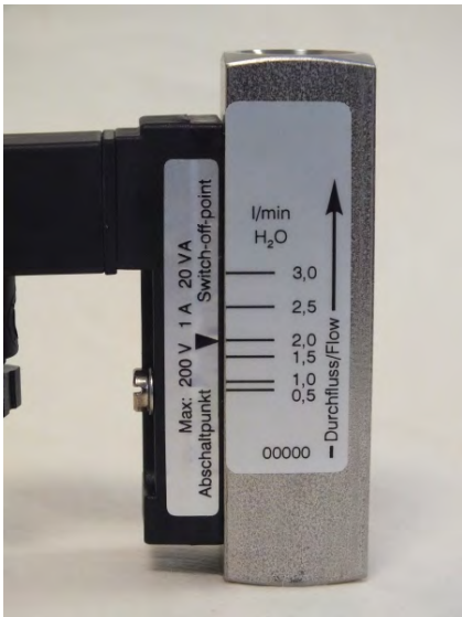
Fig. 33: Reading-off the flow value (example scale)
