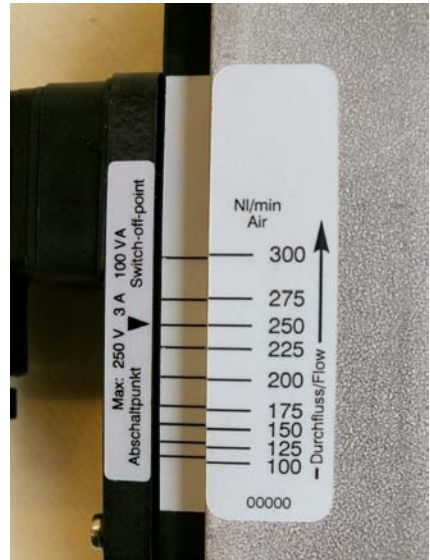
Fig. 4: Switch point adjustment scale SW-02
