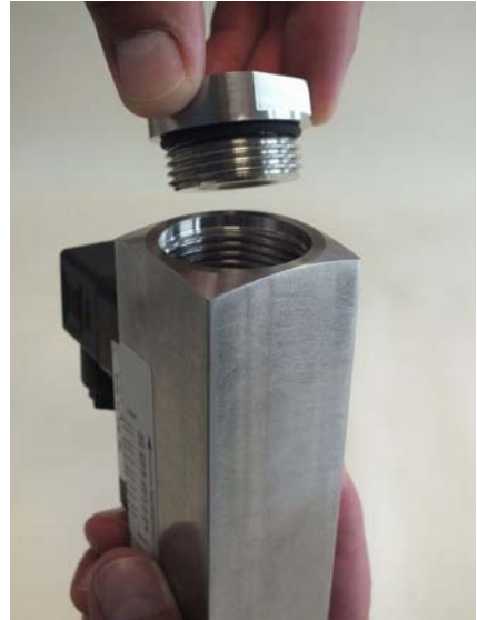
Fig. 34: Remove the process connection (outlet)
