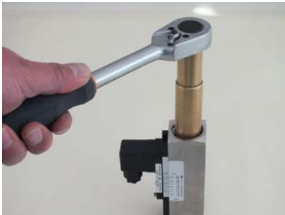
Fig. 54: Seat threaded ring (outlet)
