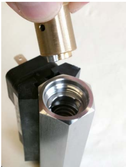
Fig. 33: Insert threaded ring insertion tool (outlet)
