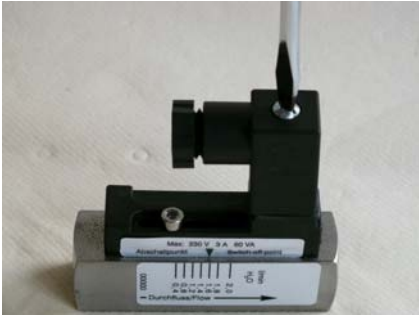
Fig. 49: Loosen female socket
