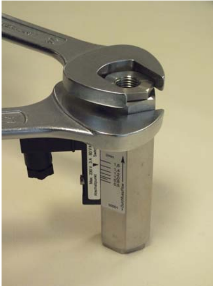
Fig. 34: Loosen process connection (outlet)
