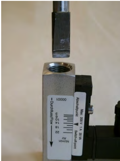
Fig. 39: Insert threaded ring insertion tool (inlet)
