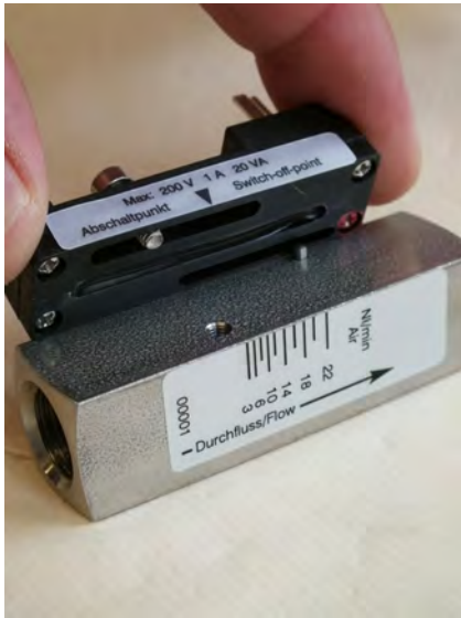
Fig. 52: Remove switch contact
