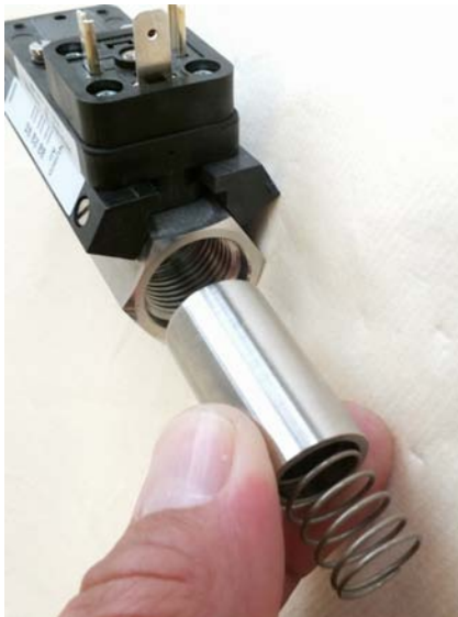
Fig. 36: Remove inner parts
