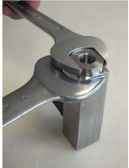
Fig. 50: Tighten process connection (inlet)
