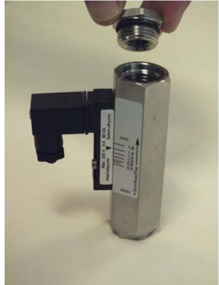
Fig. 35: Remove the process connection (outlet)
