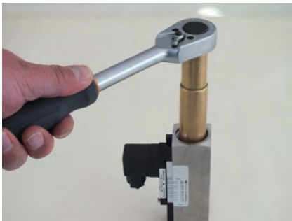
Fig. 37: Loosen threaded ring (outlet)
