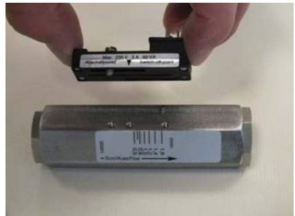
Fig. 57: Remove switch contact
