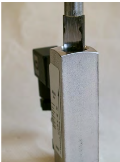
Fig. 47: Seat threaded ring (outlet)
