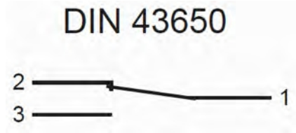
Fig. 15: Switch position under no-flow condition
