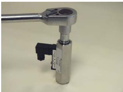
Fig. 37: Loosen threaded ring (outlet)
