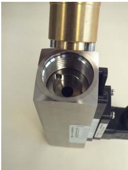
Fig. 35: Insert threaded ring insertion tool (outlet)
