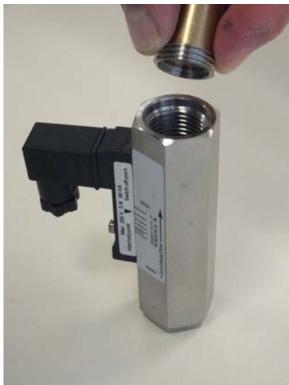
Fig. 38: Remove threaded ring (outlet)
