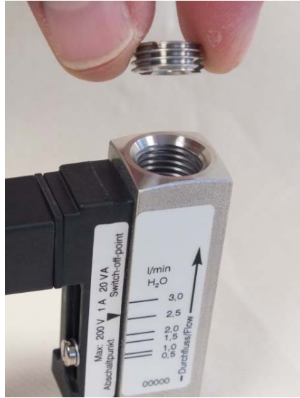
Fig. 46: Insert threaded ring (outlet)
