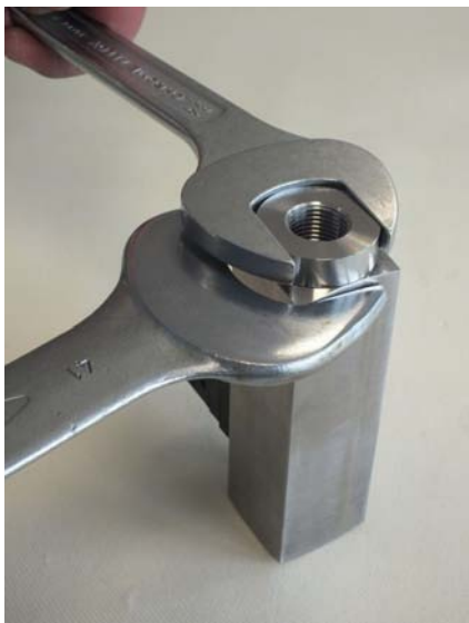
Fig. 40: Loosen process connection (inlet)
