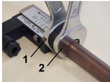
Fig. 10: Screw in the device
