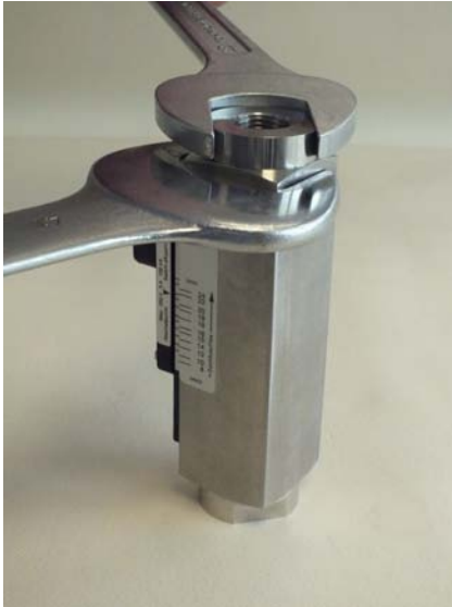
Fig. 33: Loosen process connection (outlet)
