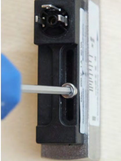
Fig. 32: Loosen the set screw
