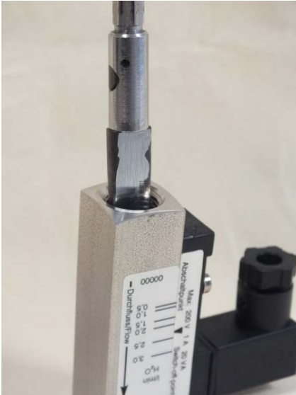
Fig. 40: Loosen threaded ring (inlet)
