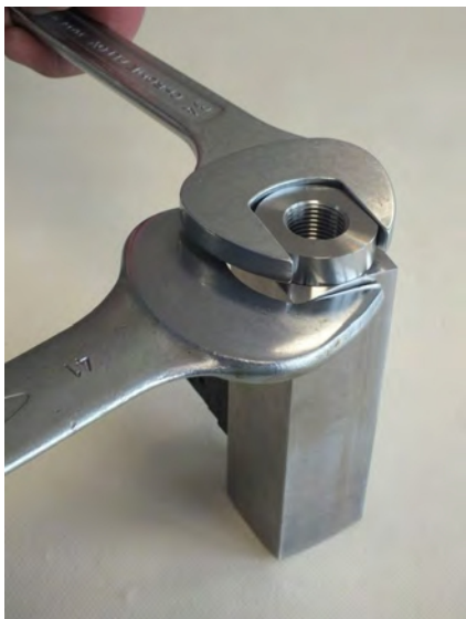
Fig. 51: Tighten process connection (inlet)
