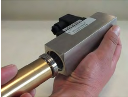
Fig. 48: Insert threaded ring (inlet)
