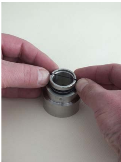
Fig. 39: O-ring (glass buffer)
