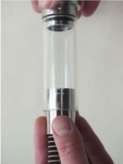
Fig. 37: Remove float and spring
