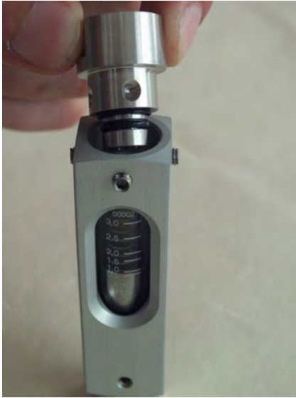
Fig. 35: Remove the process connection (outlet)
