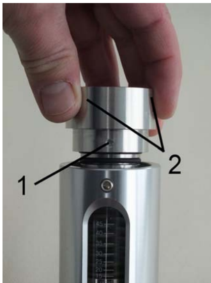
Fig. 48: Position the process connection (outlet)
