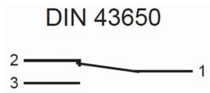
Fig. 14: Switch position under no-flow condition
