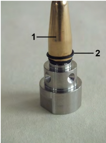
Fig. 40: O-ring (Glass buffer)
