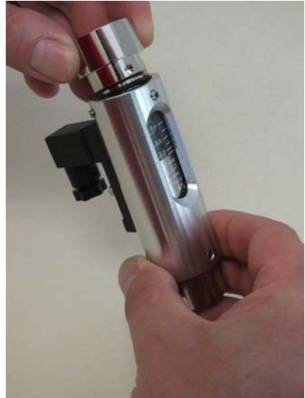
Fig. 34: Remove the process connection (outlet)
