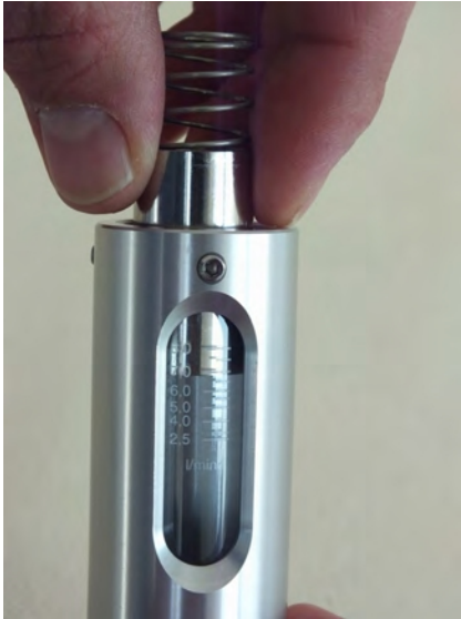
Fig. 48: Insert float and inner parts
