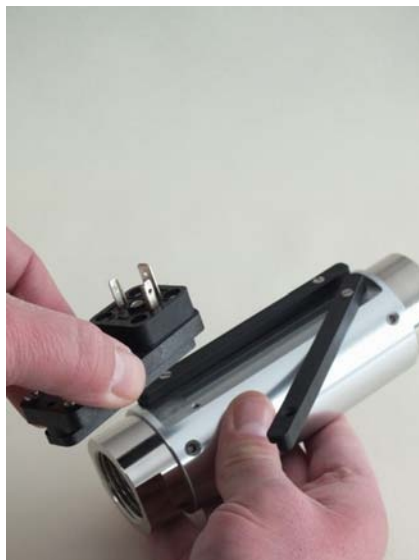
Fig. 56: Remove switch contact
