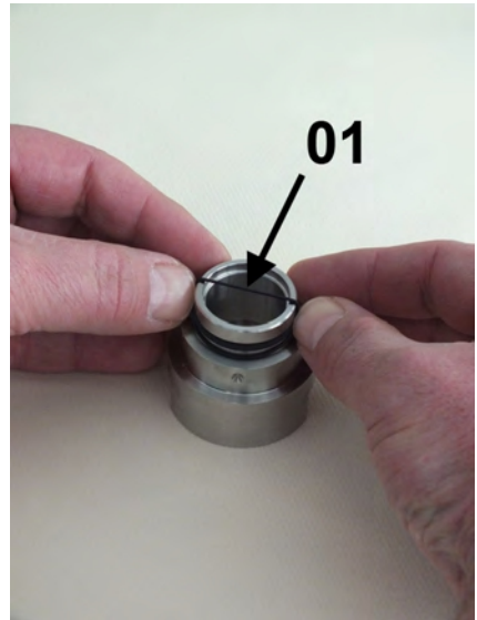
Fig. 40: O-ring (Glass buffer)
