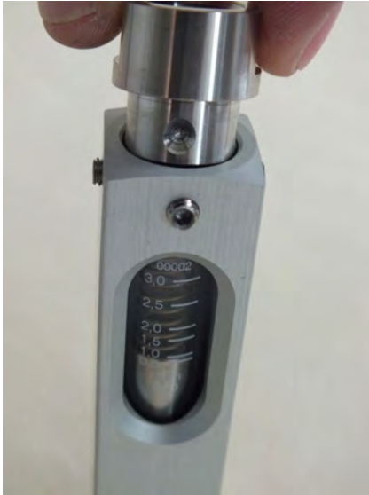
Fig. 49: Position process connection (outlet) in device housing
