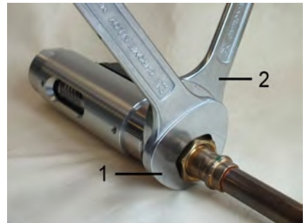
Fig. 11: Screw in the device
