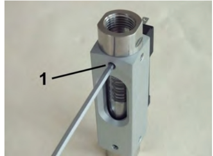
Fig. 50: Tighten hex socket screws
