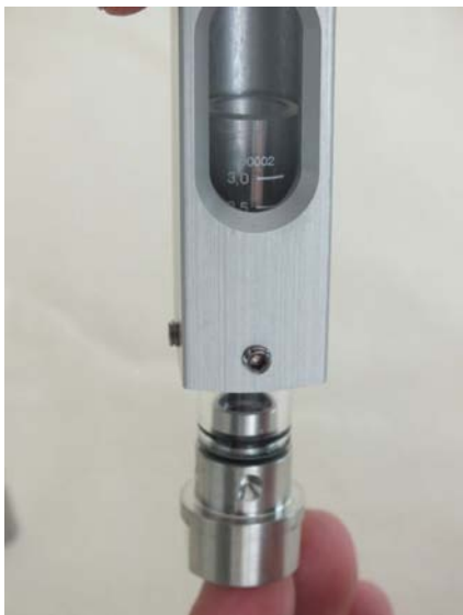
Fig. 44: Insert process connection into device housing
