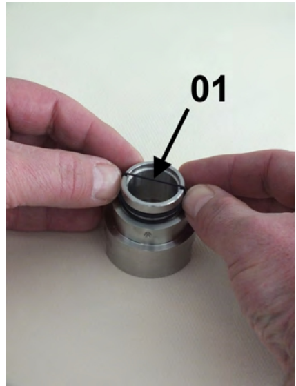
Fig. 40: O-ring (Glass buffer)
