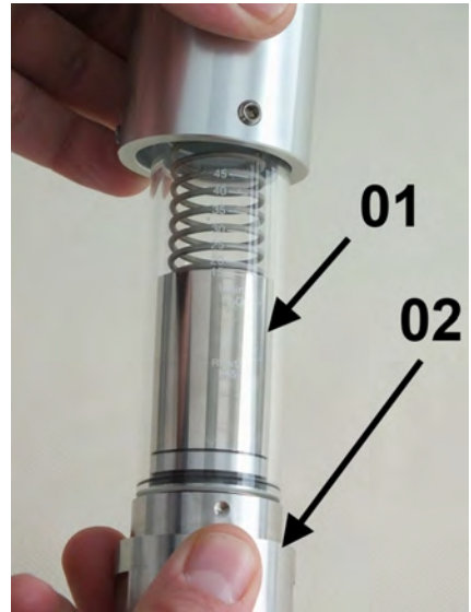
Fig. 37: Remove inner section
