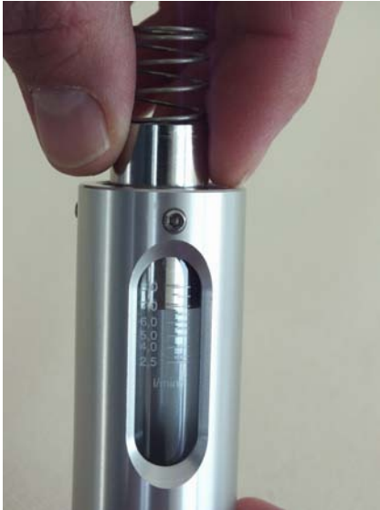
Fig. 47: Insert the inner parts
