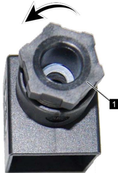
Fig. 22: Loosen the screw connection
