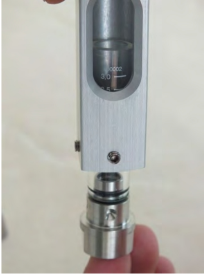
Fig. 45: Insert the process connection into the device housing
