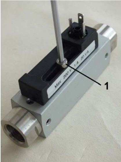
Fig. 53: Remove set screw
