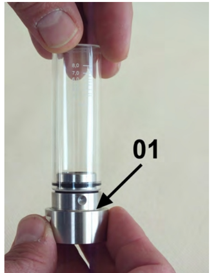
Fig. 43: Process connection (inlet) in sight glass
