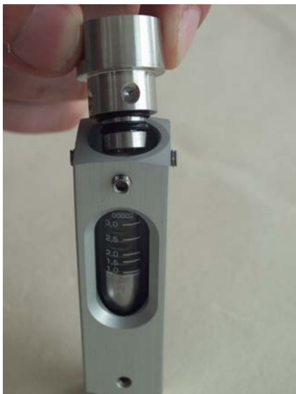
Fig. 34: Remove the process connection (outlet)
