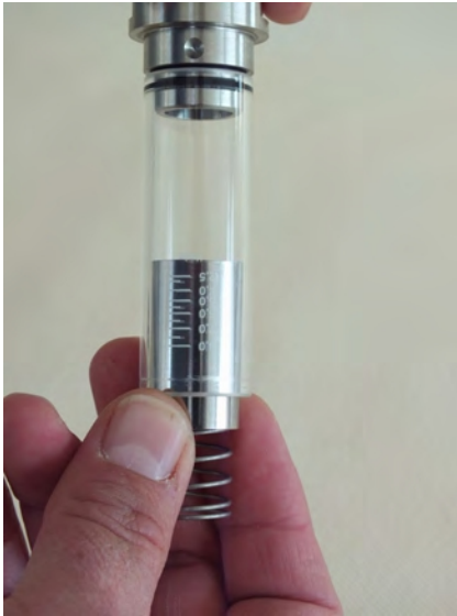
Fig. 38: Remove float, magnets and spring
