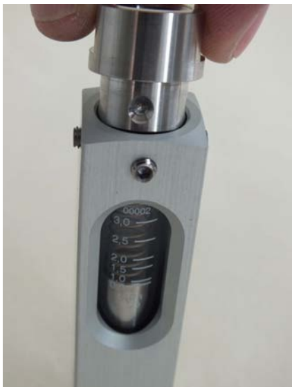
Fig. 48: Position the process connection (outlet)
