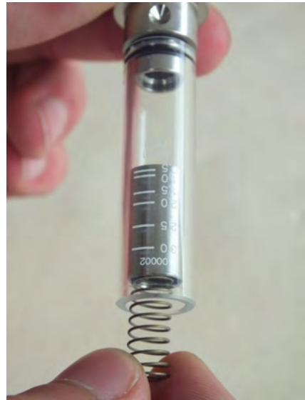
Fig. 38: Remove float, magnets and spring
