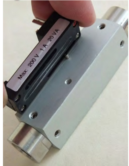
Fig. 55: Remove switch housing
