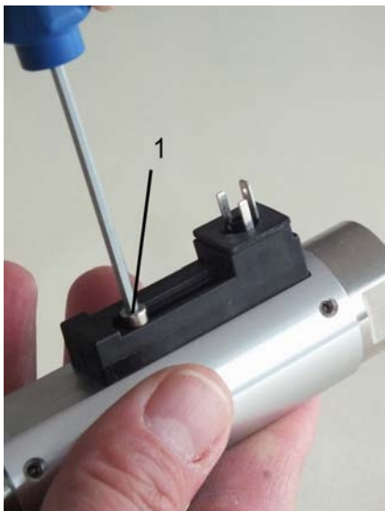
Fig. 53: Remove set screw
