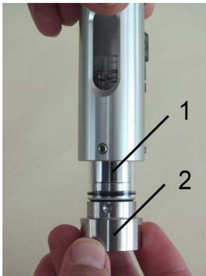
Fig. 36: Remove the inner parts
