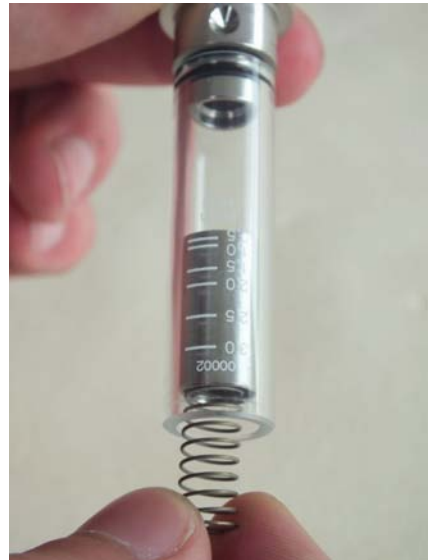
Fig. 37: Remove float and spring
