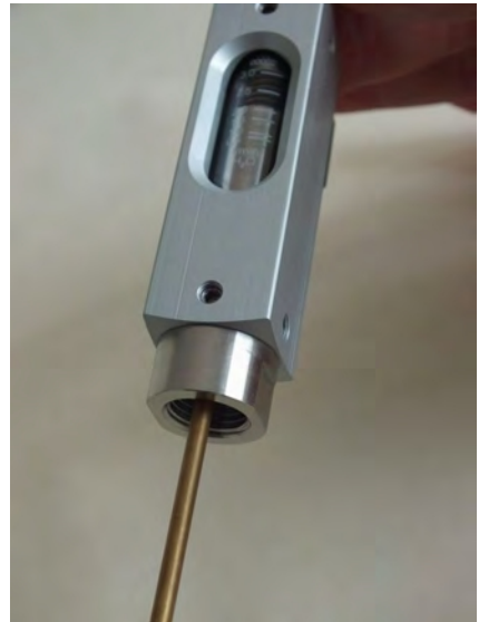
Fig. 51: Check for ease of movement
