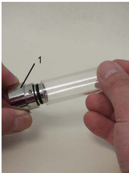
Fig. 42: Process connection (inlet) and sight glass
