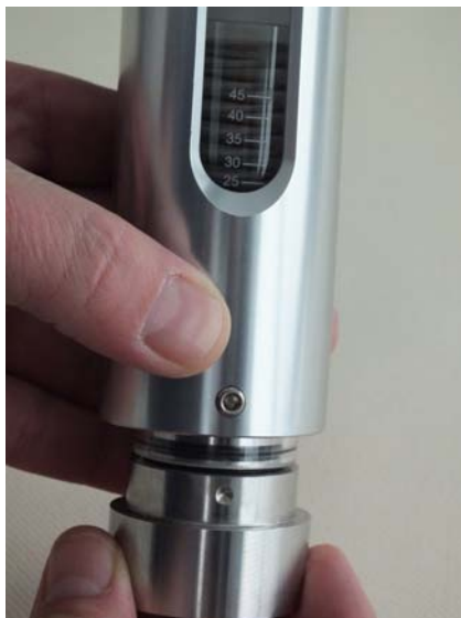
Fig. 44: Insert the process connection into the device housing
