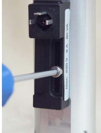
Fig. 31: Loosen set screw
