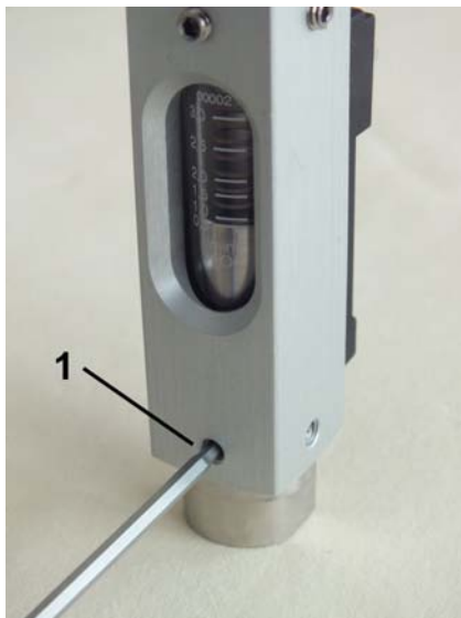
Fig. 45: Secure the process connection (inlet)
