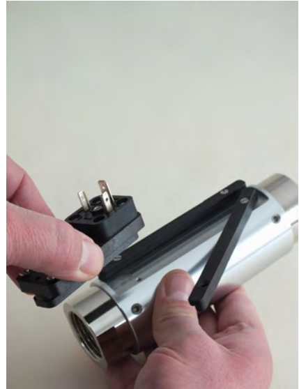
Fig. 57: Remove switch contact
