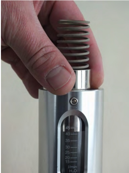
Fig. 48: Insert float and inner parts
