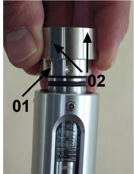
Fig. 49: Position process connection (outlet) in device housing
