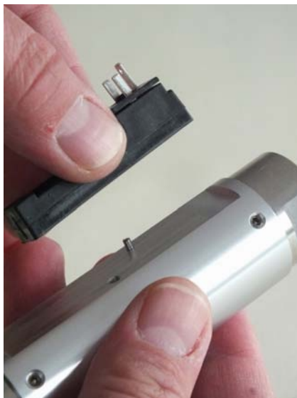
Fig. 54: Remove switch contact
