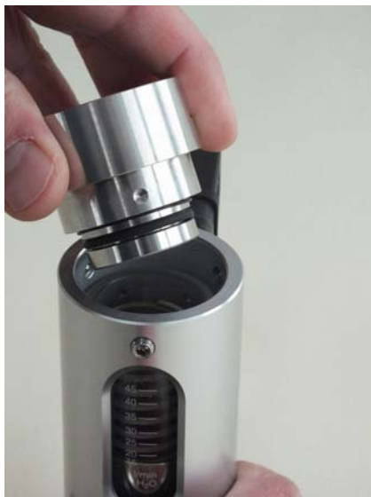
Fig. 34: Remove the process connection (outlet)
