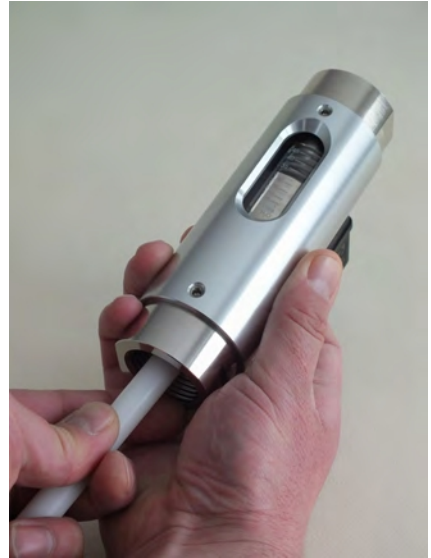
Fig. 51: Check for free movement
