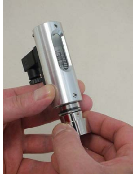
Fig. 44: Insert process connection into device housing
