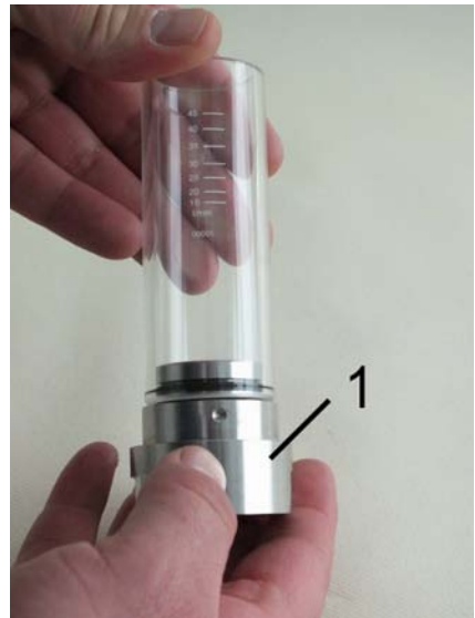
Fig. 42: Process connection (inlet) and sight glass
