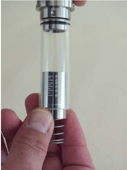
Fig. 37: Remove float and spring
