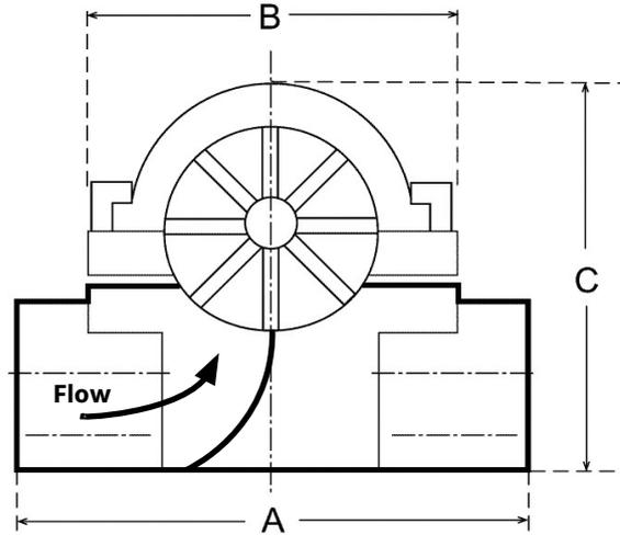
**Attention:** Mounting in direction of flow, as indicated with an arrow on the device.
